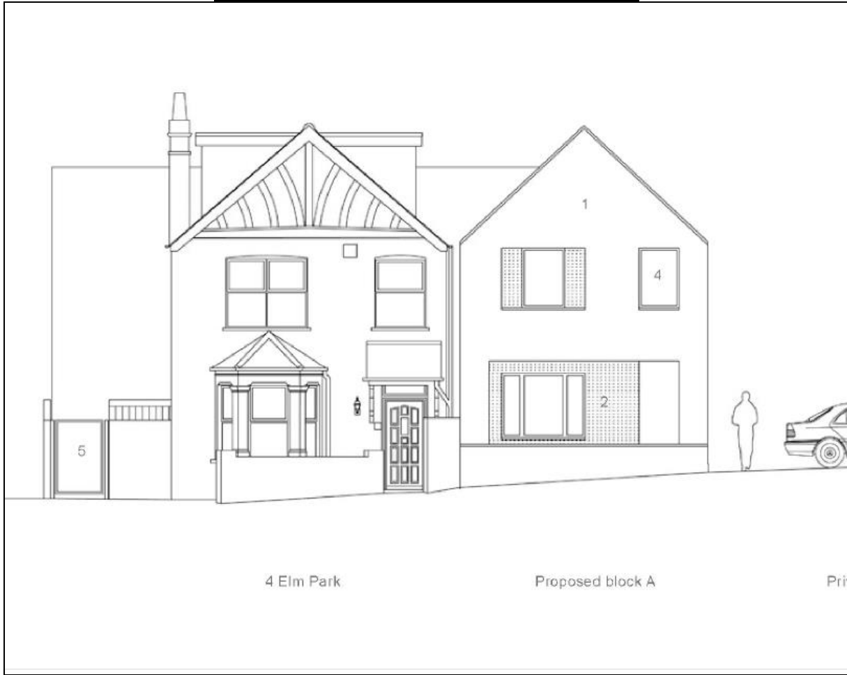
Proposed Front Elevation
